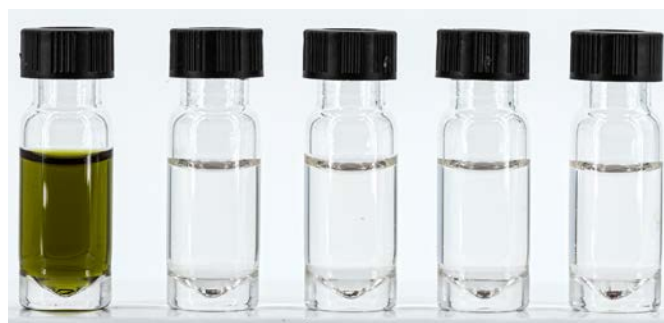
Figure 4: Visible matrix reduction: cannabis extract, competitor 1, competitor 2, competitor 3, MACHEREY-NAGEL (from left to right).
