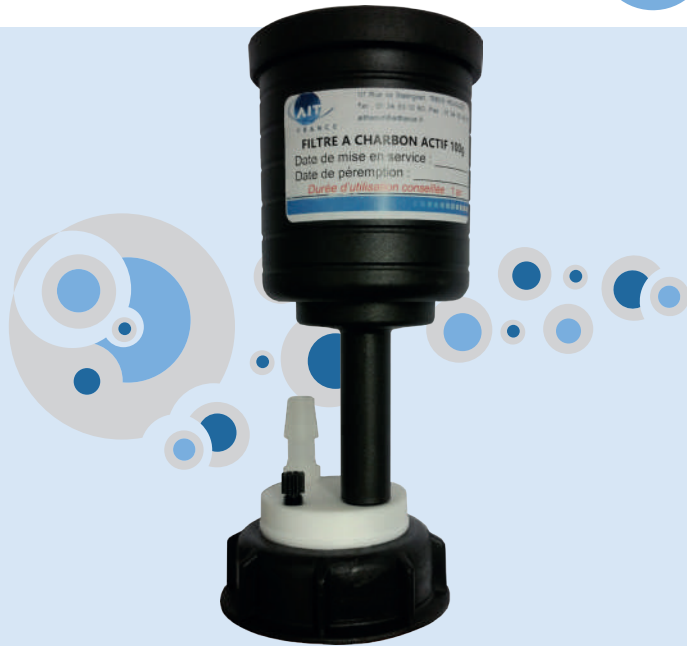
SW60-5-C-1L : 5 entries 1/8", 1 threaded barbed fitting and charcoal cartridge emplacement
