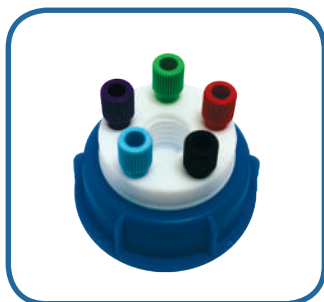
SWB-5-C : 5 entries 1/8" and charcoal cartridge emplacement
