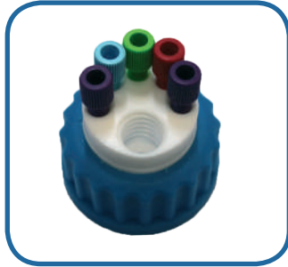
SW45-5-C : 5 entries 1/8" and charcoal cartridge emplacement
