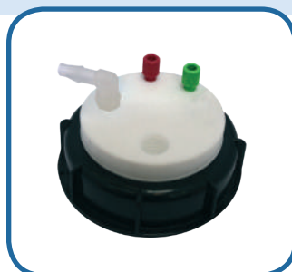
SW90-2-C-1L : 2 entries 1/8", a charcoal cartridge emplacement and 1 threaded barbed fitting
