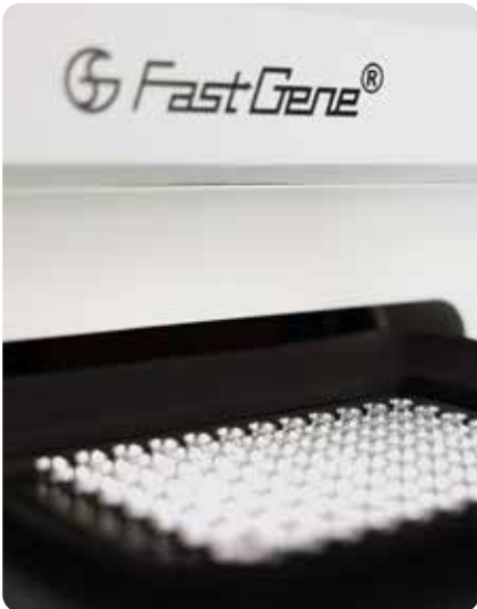
With the multiplex function, the FastGene® qFYR can discriminate up to four different targets in a single reaction well.
