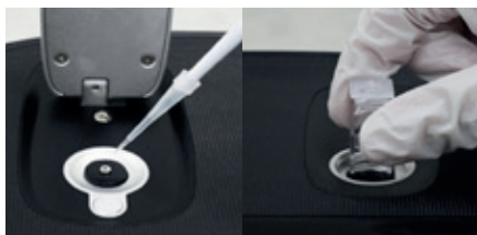
The FastGene® NanoSpec combines a microvolume drop reader with a cuvette reader.
