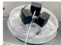
The grippers automatically adjust to the tube diameter and begin the screwing or unscrewing process.
