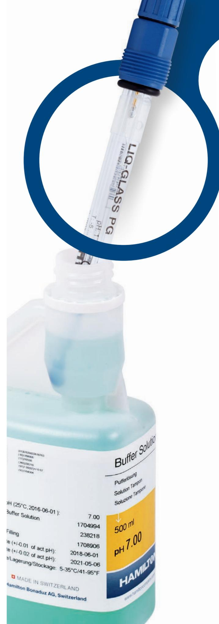
located in the inner buffer the other in the reference electrolyte. Most pH electrodes show nearly linear behavior in the measuring range of pH 0 to 14. Therefore, a pH electrode is calibrated with the help of two buffer solutions with exactly determined pH values, for example pH 4.01 and 7.00. Based on these two measurement points, a calibration curve is obtained by linear interpolation and extrapolation.
