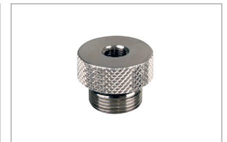
187100-25 Oil mist outlet (optional) It is used to exhaust the oil mist out of a room by connecting an optional hose barb (Thread 1/8 PT) and a proper tube.
